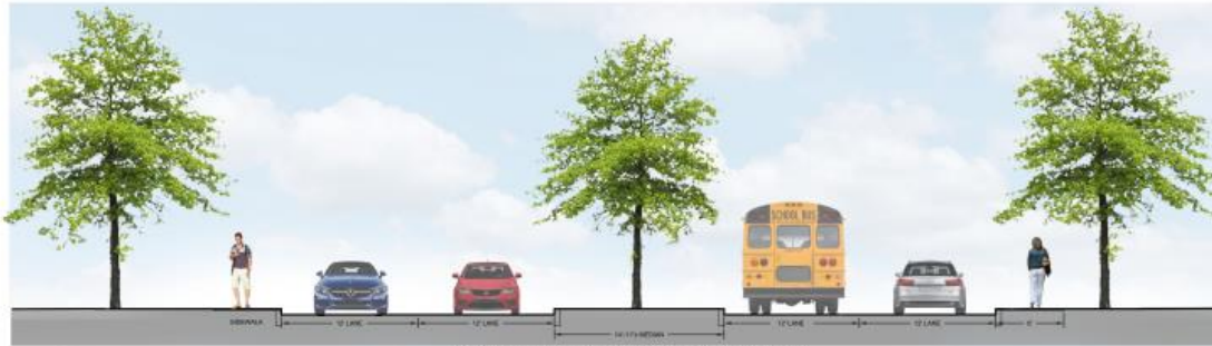
PROPOSED MONTEITH DRIVE SECTION A - A' SCALE: 1" = 5'
